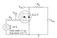
Fig. 13 - Switching Time Test Circuit
