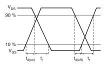
Fig. 14 - Switching Time Waveforms
