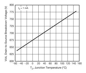
Fig. 11 - Temperature vs. Drain-to-Source Voltage
