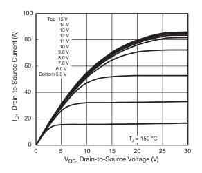
Fig. 2 - Typical Output Characteristics,  $T_C = 150$  °C
