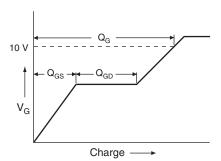
Fig. 17 - Basic Gate Charge Waveform
