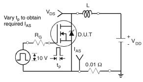
Fig. 15 - Unclamped Inductive Test Circuit
