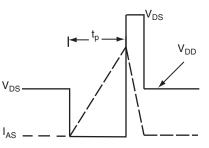
Fig. 16 - Unclamped Inductive Waveforms
