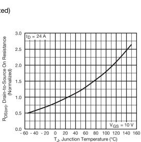
Fig. 4 - Normalized On-Resistance vs. Temperature
