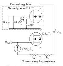
Fig. 18 - Gate Charge Test Circuit
